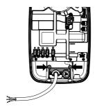
Use the provided 2 M6x14 (Torque 2.5Nm) screws to secure the charger unit to the wall bracket through the clearance holes and tapped holes inside of the mounted charger.
