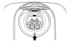
3) Use the provided 1 M4x8 screw (Torque 1.2Nm) to secure the socket lid frame to the charger socket frame.
