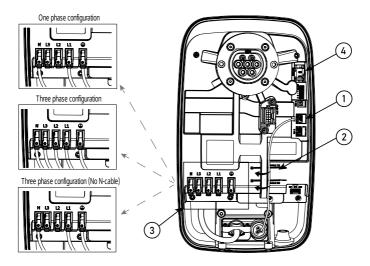
2) Connect each cable to its corresponding cable slot using the locking system: lift the slot lid, insert the cable and close the slot lid.
