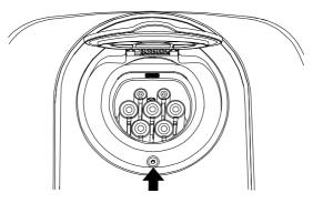
3) Use the provided 1 M4x8 screw (Torque 1.2Nm) to secure the socket lid frame to the charger socket frame.
