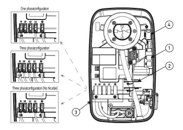
Connect each cable to its corresponding cable slot using the locking system: lift the slot lid, insert the cable and close the slot lid.
