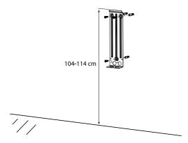
Note: Use proper levelling tool to make sure that the wall bracket is levelled.
