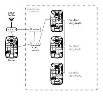
Required equipment for installation: 4port switch installed between Master and first satellite.
