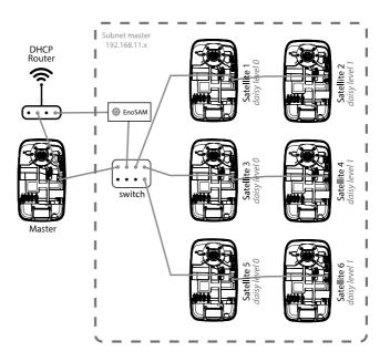
Required equipment for installation: #port switch installed between Master and first satellite.
